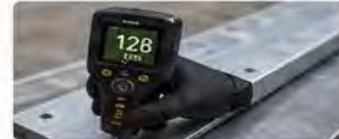
Coating Thickness Measurement Ensuring coating compliance with project requirements.
